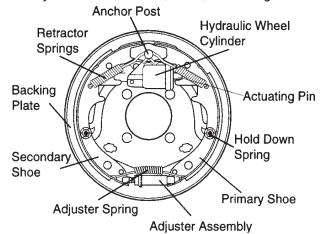
Figure 55. Hydraulic Brake Components
